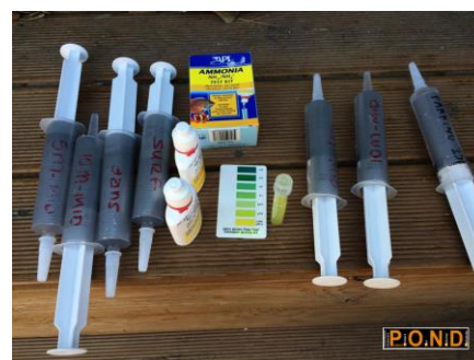
Image 3: Ammonia NH 3 – Test during actual measurement.
