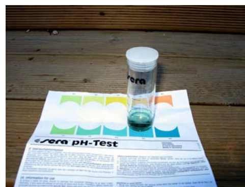
Image 3: Sera pH – Test during actual measurement.
